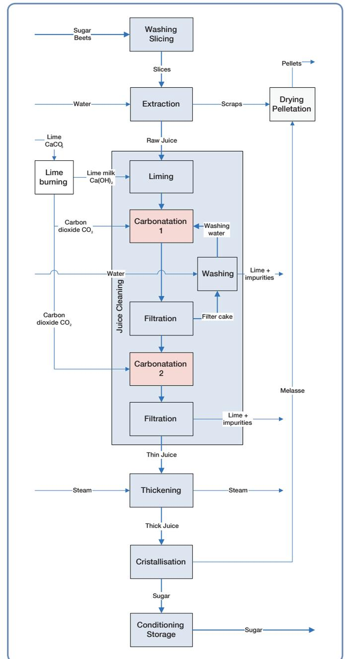
Figure 1: Simplified scheme of the sugar production from sugar beets. This application note focuses on the carbonatation (red).
