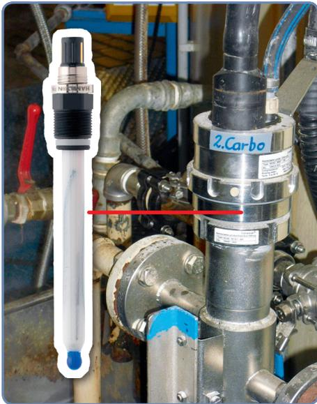
Figure 2: pH sensor mounted in the second carbonatation
