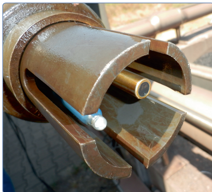
Fig. 2: VisiFerm DO Arc and Polilyte Plus ORP Arc sensors in a housing.
