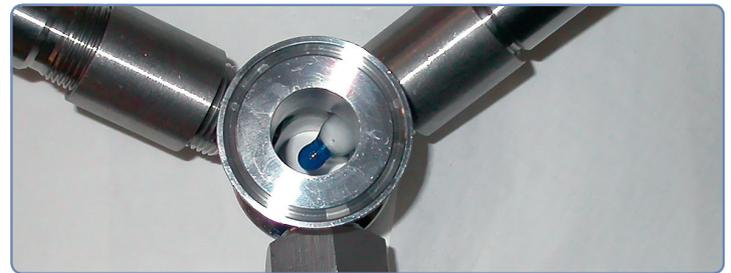
Figure 2: DO sensor (left), pH sensor (right) and sample port (in front) mounted between static mixer modules of the PFR
