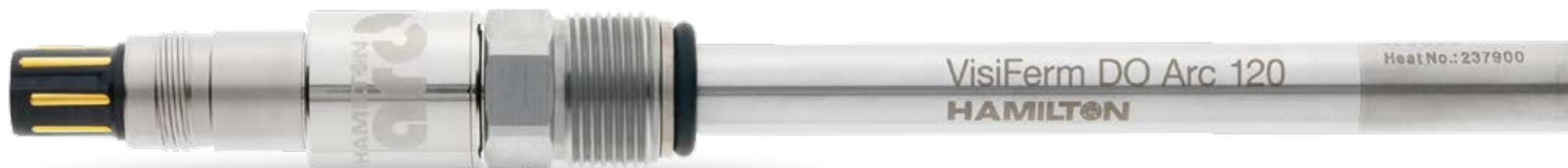
The VisiFerm DO is the first optical oxygen sensor with integrated opto-electronics, having the full functionality of a measuring device with self-diagnostics. It is steam sterilizable, autoclavable and CIP compatible. The VisiFerm requires less maintenance than a classical oxygen sensor as it does not have a mechanically sensitive membrane or a corrosive electrolyte.
