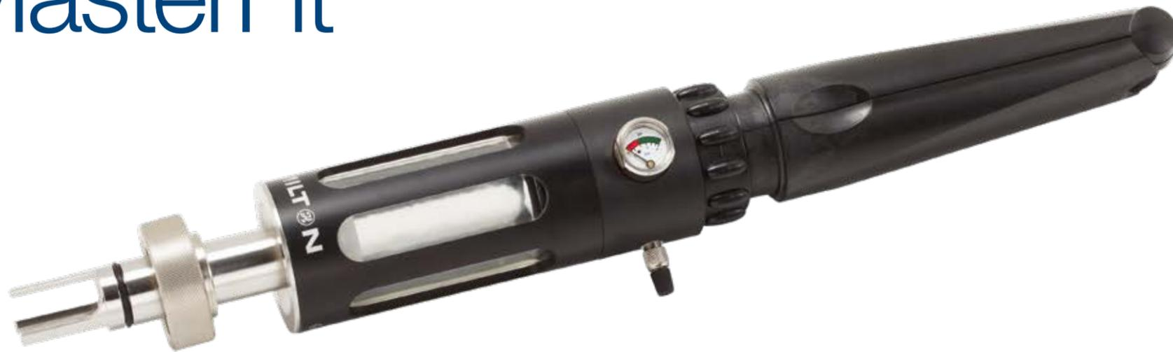
The MasterFit is a housing for pressurizable pH sensors like the ChemoTrode types. The pressurization ensures a constant outflow of electrolyte. This helps to prevent clogging of the diaphragm and poisoning of the electrolyte. The MasterFit can be used in a huge variety of applications mainly in the chemical industry.
