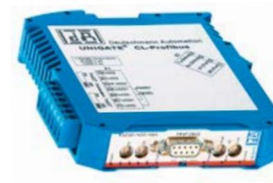
The Deutschmann Unigate® CL Module converts the Modbus protocol of the Arc and VisiFerm DO sensors into the Profibus DP protocol. All Arc parameters DO, pH, ORP and conductivity are supported. The conversion script is pre-installed.
