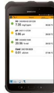
This mobile device empowers the operator to monitor measurement values, calibrate Arc sensors and configure various parameters with a unified user interface for pH, DO, Conductivity and ORP. The Arc View Mobile device is based on the Samsung Galaxy Tab Active tablet and comes pre-configured with the ArcAir application, app blocker application, power supply cable, instruction manual and Hamilton quick guide.
