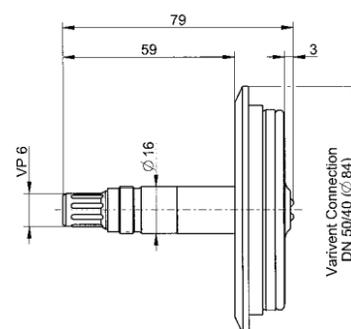
The Conducell 4UxF sensors are suited for measurements in hygienic applications. All wetted parts are FDA-approved, can be cleaned easily and withstand CIP cleanings and autoclavations. The sensors show a very good linearity over a broad measuring range. They are available with different process connections such as BioConnect® (BC) or Varivent®.
