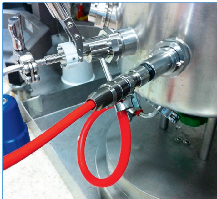
Figure 1: Installation of VisiFerm DO in a bioreactor in R&D lab.
