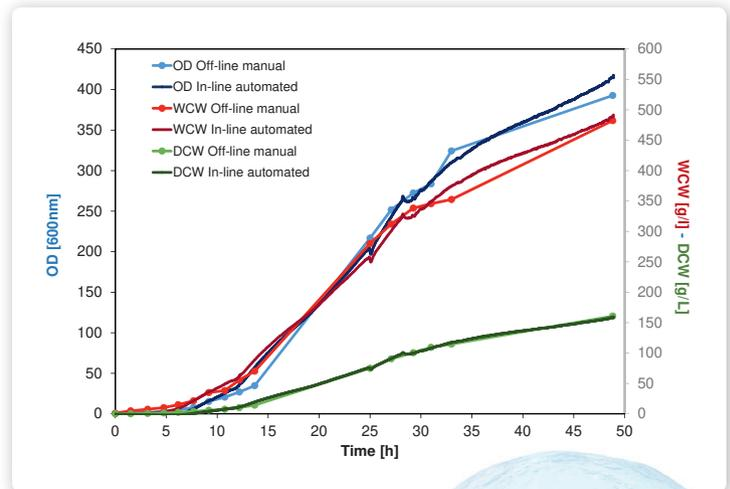
Figure 2: In-line turbidity versus off-line cell density measurements. The darker lines without dots represent the Dencytee in-line automated measurements. The lighter lines with dots represent TCD measurements from manual off-line reference methods.
