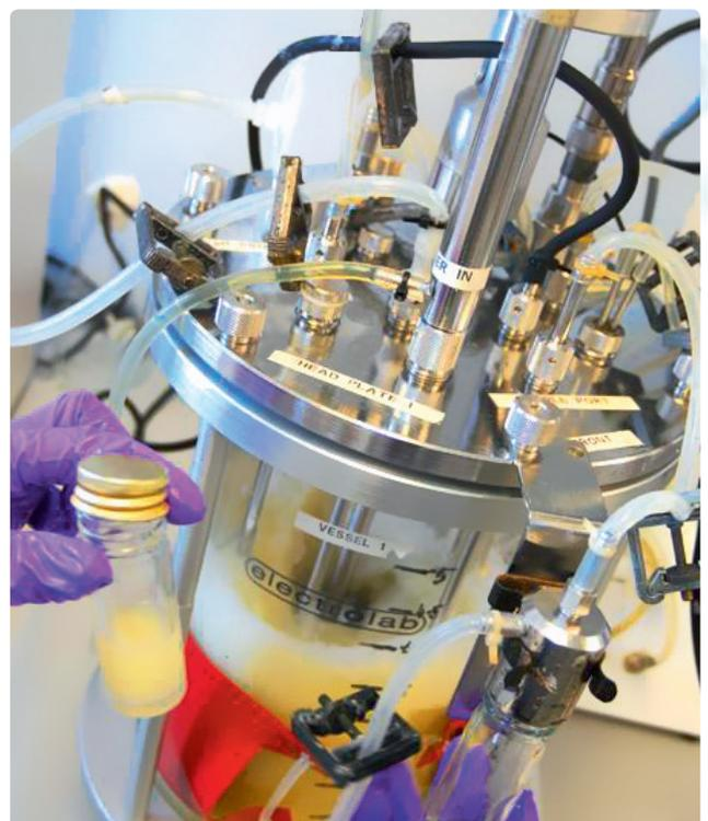
Figure 1: 5 L Electrolab Biotech Ltd bioreactor used for scale-up and scale-down studies.
