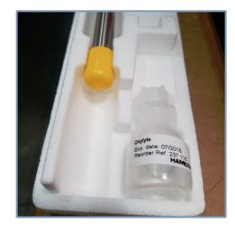
electrolyte provided with the sensor packaging has a shelf life of 2 years. If the electrolyte has expired prior to initial usage contact Hamilton for replacement solution. Electrochemical Dissolved Oxygen products include:
