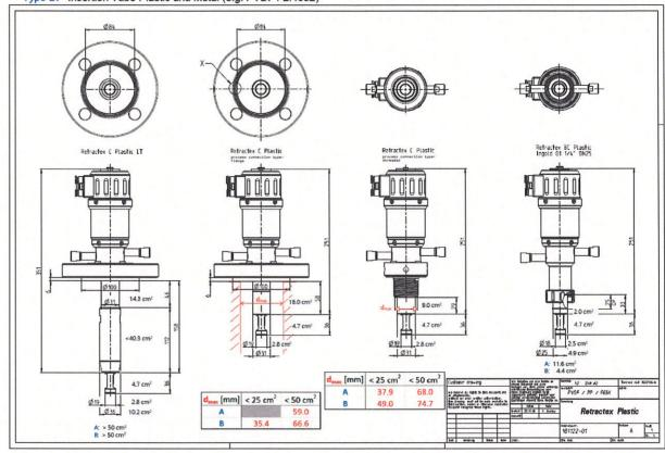
The drawing shows the correlation between the mounting situation and the diameter (flange or shaft) of the exposed plastic surface for
